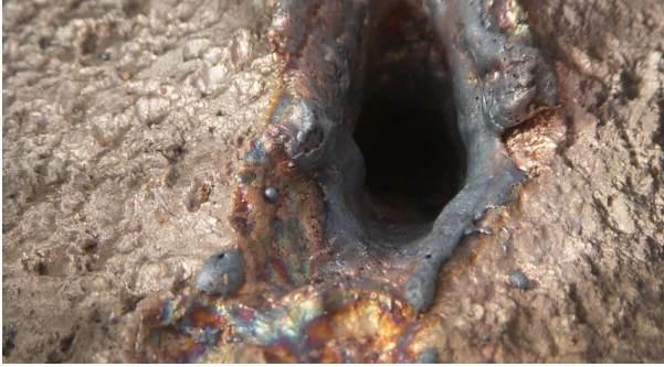
Figure 17: Penetration Test on Steel Target
